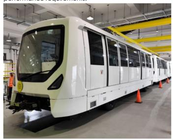
Subject to the necessary approvals from the Land Public Transport Agency (APAD) and Ministry of Transport (MOT), the Aerotrain project has to undergo 80 critical tests, including the Static, Dynamic, Interface and System Integration Tests.
